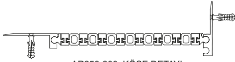
AR259-200 KÖŞE DETAYI AR259-200 CORNER DETAIL
